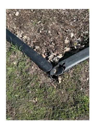
• Play area plastic edging with multiple components cracked with metal exposed.
